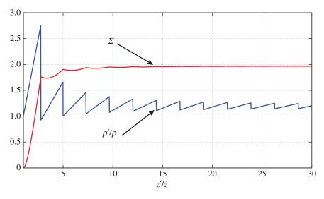
**Figure 4.** For given values of slab impedance  $z' \ge z$  and a/c = 1, the blue curve shows the value of slab density  $\rho'$  which minimizes the IE of equation (4.15). The red curve is the corresponding minimal value of  $\Sigma$ . (Online version in colour.)
