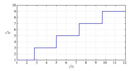
**Figure 3.** The curve shows the value of slab wave speed c' which minimizes the IE of equation (4.15) for given values of slab impedance  $z' \ge z$  and fixed slab thickness. (Online version in colour.)
