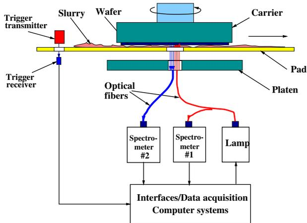
Fig. 2. A schematic of optical end-point detection systems.
