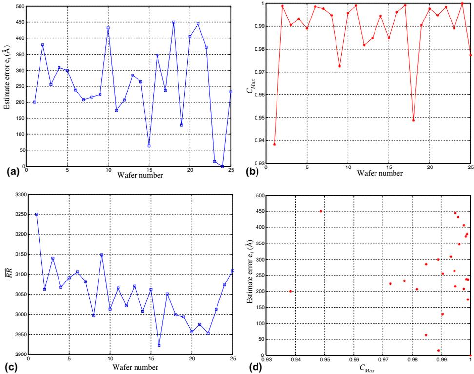
Fig. 8. Image matching results with wafer #24 (with 10-shot template and 0.9–1.1 re-scaling): (a) thickness estimate errors, (b) maximum correlation coefficients  $C_{max}$ , (c) estimate removal rate  $RR$ , (d) relationship between estimate thickness error  $e_i$  and maximum correlation coefficients  $C_{max}$ .
