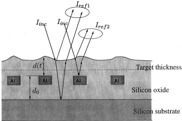
Fig. 6. Schematic of EPD optical interferometry signal path for one layer IMD film structure.
