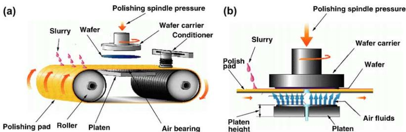
Fig. 1. (a) A schematic of Lam linear chemical–mechanical planarization systems, (b) polishing platen assembly.
