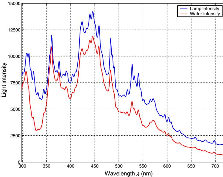
Fig. 3. An example of broadband incident and reflective intensities for an IMD CMP process.
