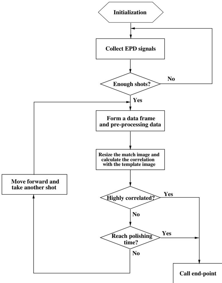
Fig. 7. A flow chart of the image matching EPD algorithm.
