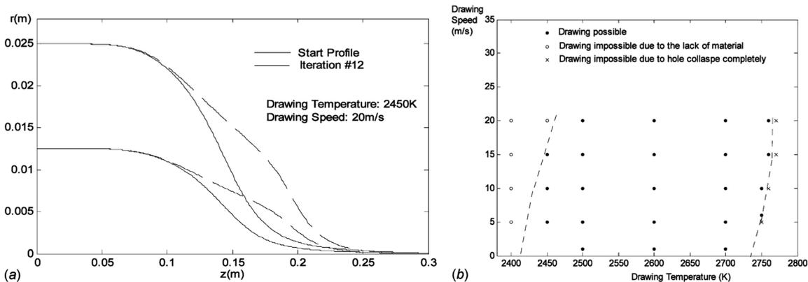
Fig. 12 Calculated neck-down profiles in hollow fiber drawing for infeasible draw conditions and the feasibility domain [52]
