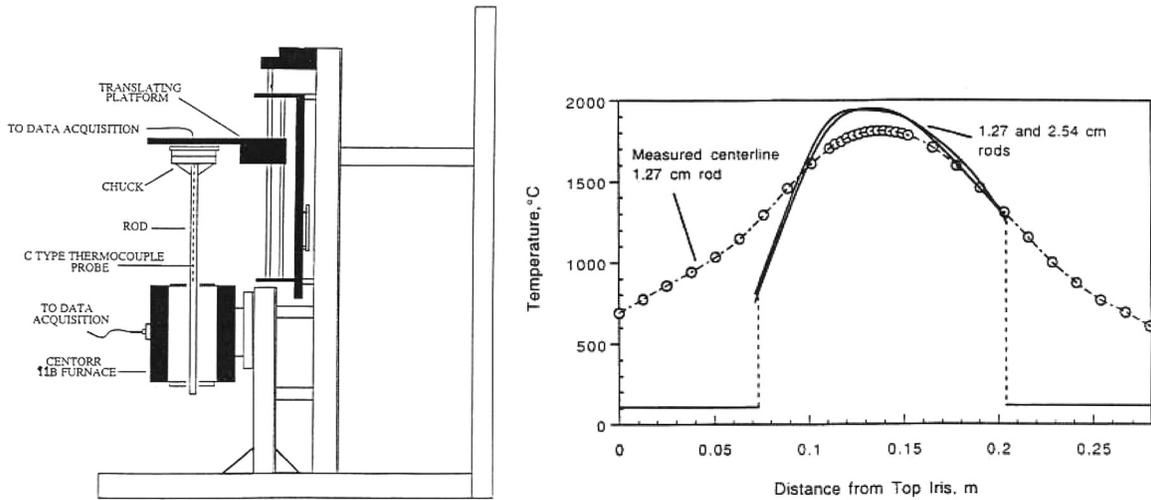
Fig. 11 Sketch of a fiber drawing furnace with an instrumented graphite rod at the center and the solution from an inverse problem to determine the furnace wall temperature distribution [50]
