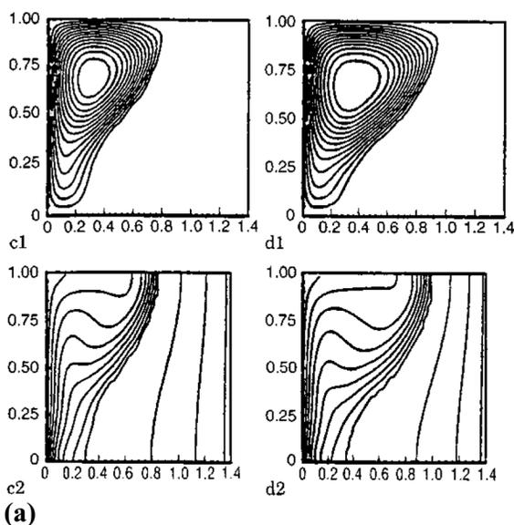
Fig. 4 (a) Streamlines (1) and isotherms (2) for melting of gallium in an enclosed region, with the left vertical boundary at a temperature higher than melting point, the right vertical boundary at a temperature lower than melting point, and the remaining two boundaries insulated, at dimensionless time  $t$  following the onset of melting of  $t = 1.5622$  and  $t = 1.9789$ . (b) Calculated streamlines in an impingement CVD reactor showing the effect of buoyancy in the center [18].
