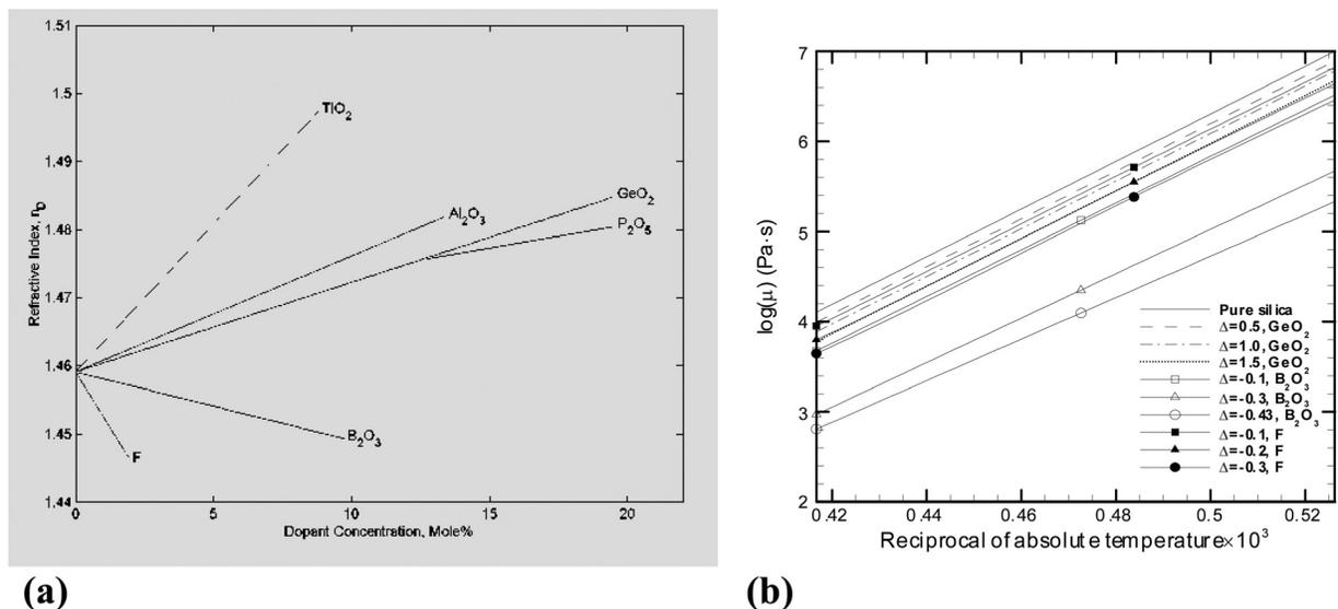
Fig. 2 Variation of silica glass properties with dopant concentration and temperature (adapted from [10–12])
