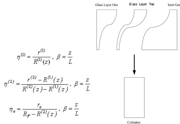
Fig. 5 Landau's transformations to convert axisymmetric complex shapes to cylindrical ones
