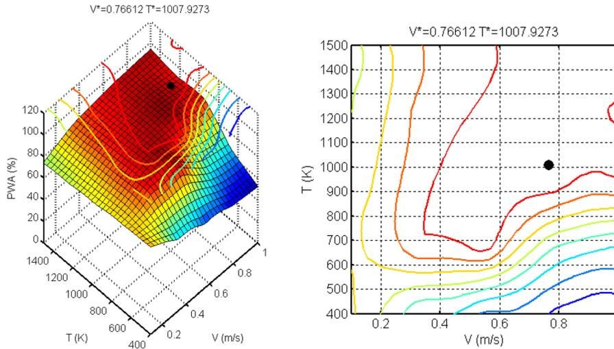
**Fig. 13** Response surface for the percentage working area (PWA) and the optimal conditions in terms of susceptor temperature and average inlet flow velocity for an impingement CVD reactor for the deposition of silicon [36,54]
