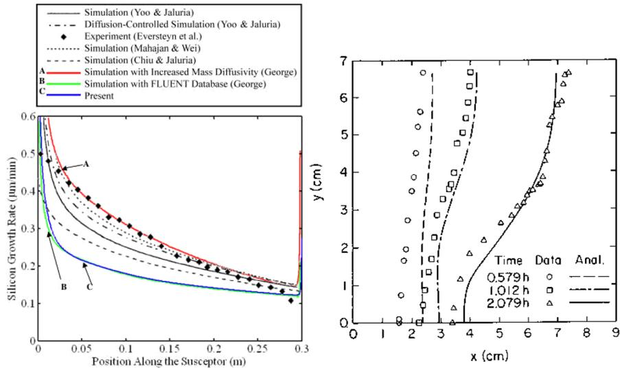
**Fig. 7 Comparison between numerical results and measurements for (a) a horizontal CVD reactor for silicon [36] and (b) melting of tin in an enclosure [18]**
