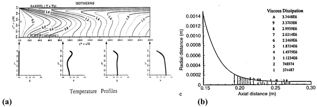
**Fig. 3 (a) Isotherms and temperature distributions in a single-screw polymer extruder [15]. (b) Viscous dissipation in the neck-down region of an optical fiber drawing process [16].**
