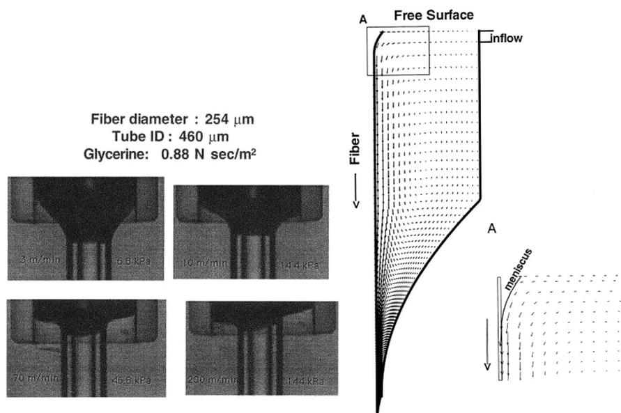
**Fig. 8 (a) Observed meniscus for different operating conditions in optical fiber coating and (b) calculations on the flow with a specified meniscus**
