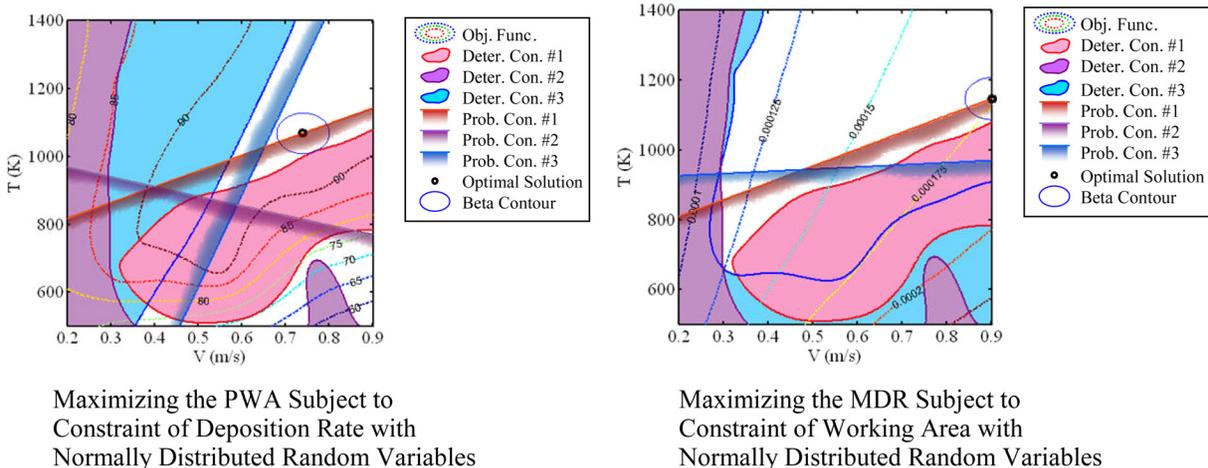
**Fig. 14** Optimization with deterministic and probabilistic constraints for normally distributed variables, indicating the optimization with variables with given uncertainties to achieve a specified level of reliability [36]
