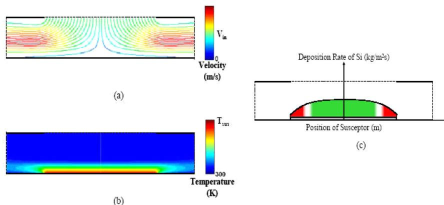
Fig. 9 Typical results on flow, temperature distribution, and deposition in a CVD reactor [36]
