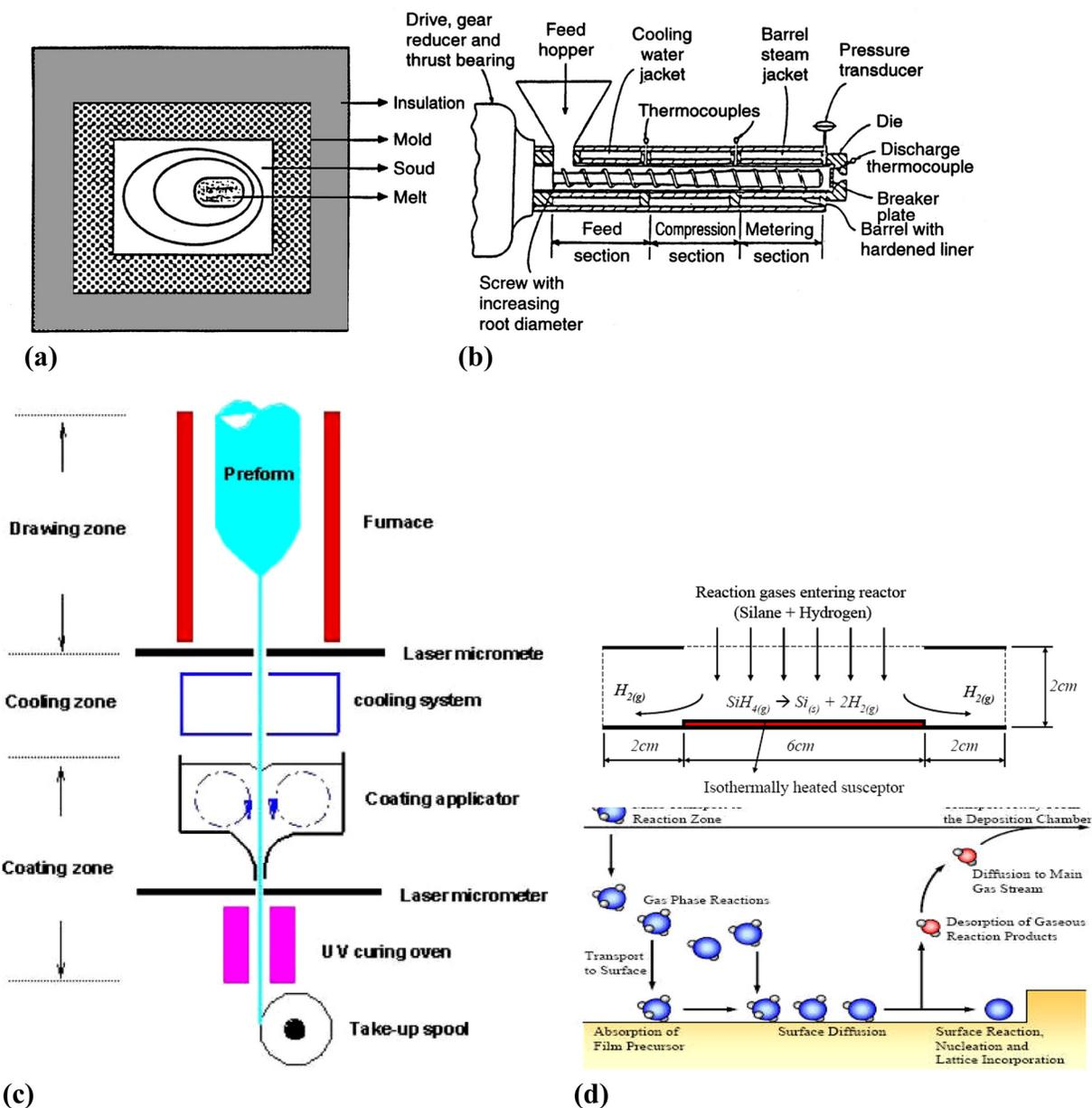
Fig. 1 Sketches of a few materials processing applications that involve significant thermal issues: (a) casting, (b) polymer single-screw extrusion, (c) optical fiber drawing, and (d) chemical vapor deposition
