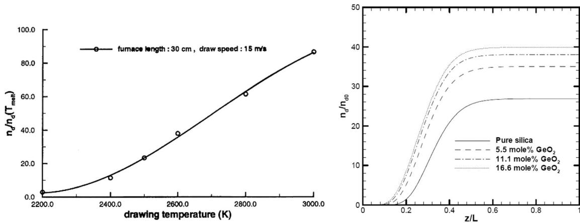
Fig. 10 Dependence of the thermally induced  $E$  defects in optical fiber drawing on furnace temperature and dopant concentration [47]
