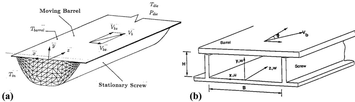
**Fig. 6** Single-screw extruder with two different channel profiles. The coordinate system is located on the barrel and curvature effects are neglected for the mathematical model.
