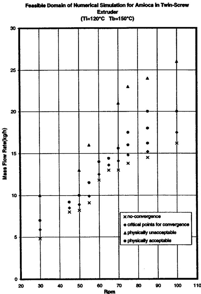
Fig. 17 Feasible domain for twin-screw extrusion of starch
