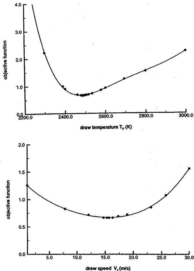
**Fig. 19 Evaluation of optimal draw temperature at a draw speed of 15 m/s and the optimal draw speed at a draw temperature of 2489.78 K, obtained in the first part, by using the golden-section search method**
