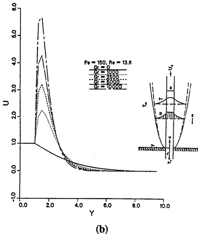
**Fig. 10 (a) Flow in the ambient fluid due to a continuously moving material; (b) dimensionless velocity ( $u/U_s$ ) distribution in the fluid due to a vertically moving heated plate with aiding buoyancy effects**
