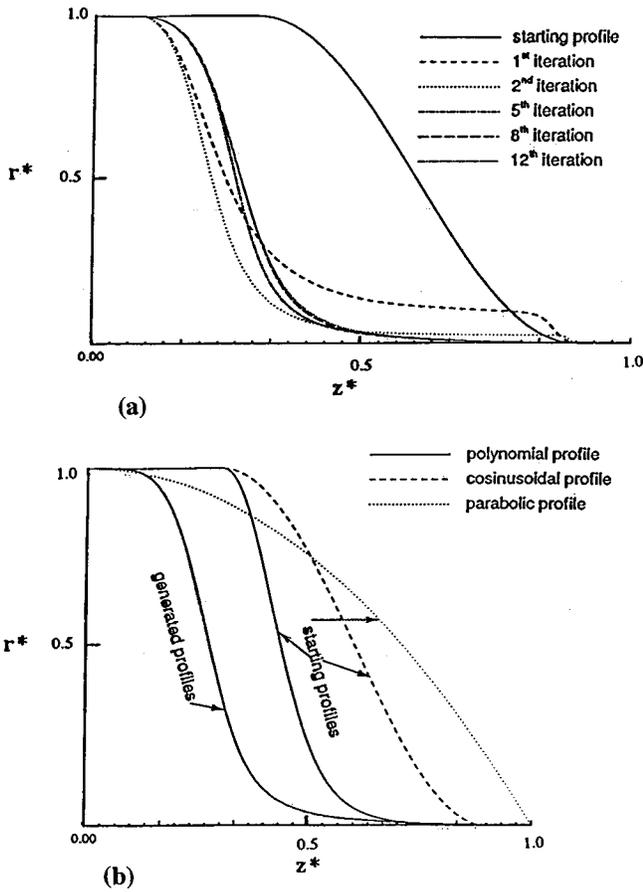
Fig. 8 (a) Iterative convergence of the neck-down profile in optical fiber drawing; (b) results for different starting profiles. Here,  $r^* = r/R$  and  $z^* = z/L$ , where  $R$  is the preform radius, and  $L$  the furnace length.
