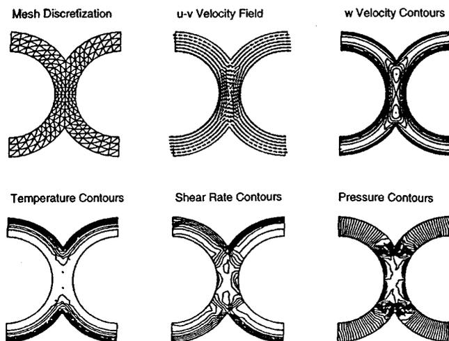
**Fig. 6 Mesh discretization for the mixing region in a corotating tangential twin screw extruder, along with typical computed results for low density polyethylene (LDPE) at  $n=0.48$ , barrel temperature,  $T_b=320^\circ\text{C}$ , inlet temperature,  $T_i=220^\circ\text{C}$ ,  $N=60$  rpm,  $q_v=0.3$**
