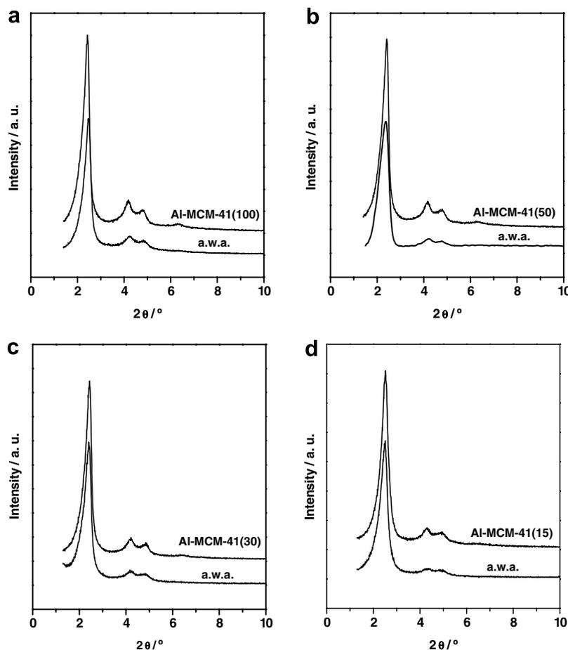
Fig. 1. Powder X-ray diffraction patterns prior to and after water adsorption (a.w.a.) of Al-MCM-41 materials with Si/Al of: (a) 100; (b) 50; (c) 30 and (d) 15.
