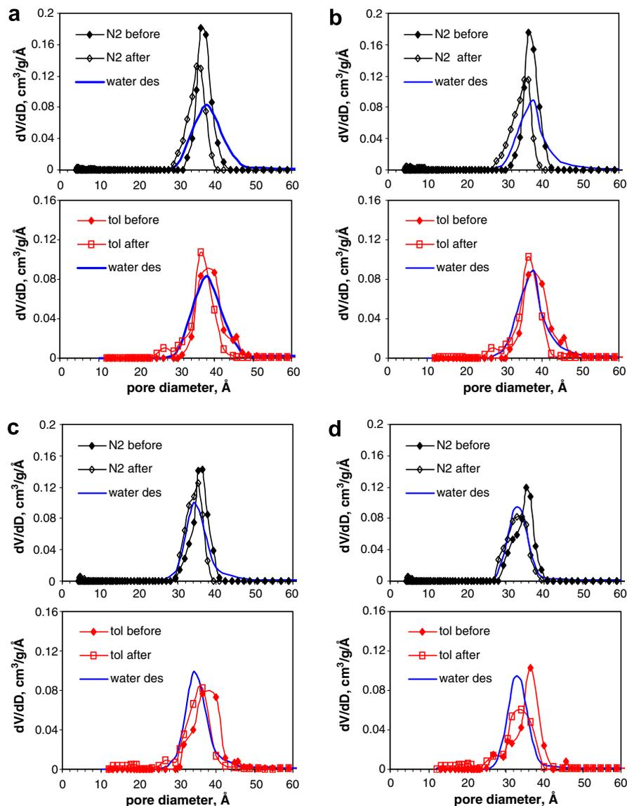
Fig. 4. Pore volume distributions prior to and after water adsorption (a.w.a) calculated from nitrogen isotherms, using NLDFT method [39] and from toluene isotherms using hybrid MC-DBdB method [40], of Al-MCM-41 materials with Si/Al of: (a) 100; (b) 50; (c) 30 and (d) 15. Also shown are pore volume distributions calculated from water desorption isotherms using DBdB method (see text).
