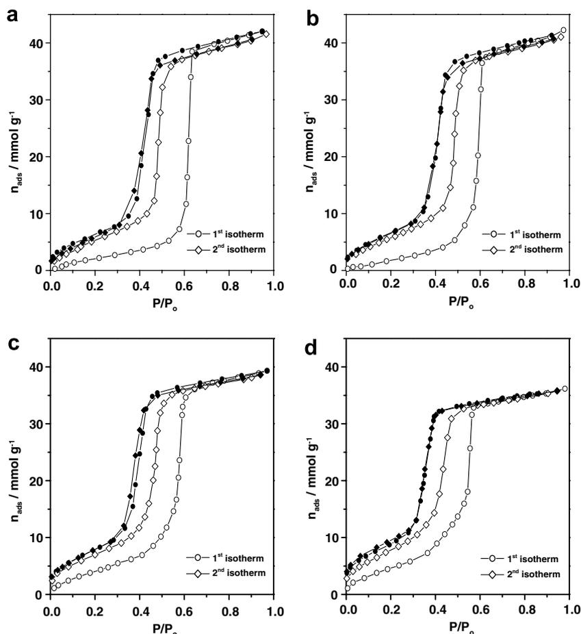
Fig. 5. Two consecutive water adsorption isotherms at 298 K on Al-MCM-41 materials with Si/Al of: (a) 100; (b) 50; (c) 30 and (d) 15 (empty symbols: adsorption, filled symbols: desorption).
