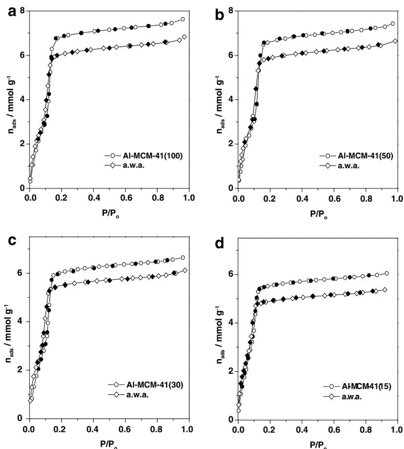
Fig. 3. Toluene adsorption isotherms at 298 K determined prior to and after water adsorption (a.w.a.) on Al-MCM-41 materials with Si/Al of: (a) 100; (b) 50; (c) 30 and (d) 15 (empty symbols: adsorption, filled symbols: desorption).
