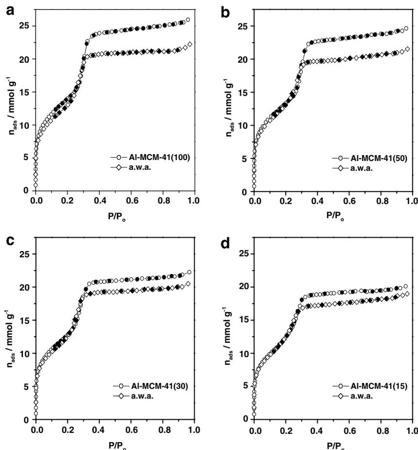
Fig. 2. Nitrogen adsorption isotherms at 77 K determined prior to and after water adsorption (a.w.a) on Al-MCM-41 materials with Si/Al of: (a) 100; (b) 50; (c) 30 and (d) 15 (empty symbols: adsorption, filled symbols: desorption).
