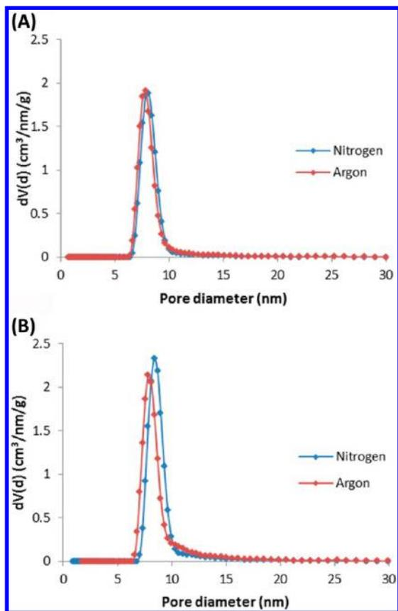
**Figure 5.** Nitrogen and argon QSDFT pore size distributions calculated from the desorption branch of the isotherms for (A) 10 nm 3DOm carbon and (B) 20 nm 3DOm carbon.
