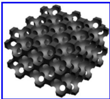
**Figure 1.** Representative three-dimensionally ordered mesoporous (3DOM) carbon structure.
