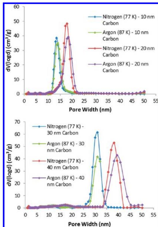
**Figure 4.** Pore size distributions calculated from the  $N_2$  (77.4 K) and Ar (87.3 K) adsorption isotherms using QSDFT methods designed for carbons with spherical mesopores.
