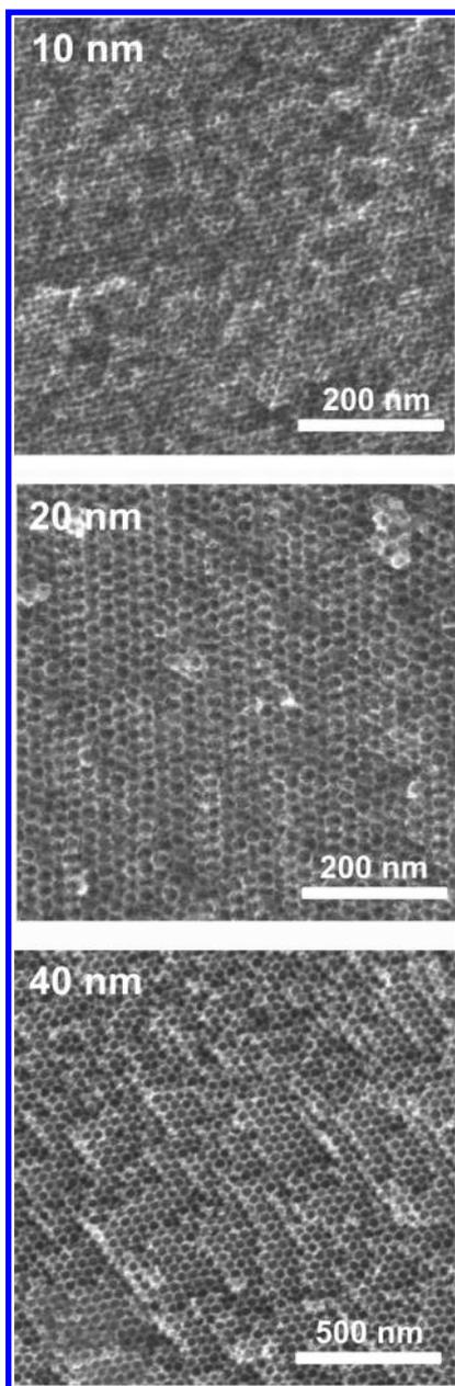
**Figure 3.** Representative SEM images of 10, 20, and 40 nm 3DOM carbons prepared by replication of colloidal crystals composed of lysine–silica nanoparticles.
