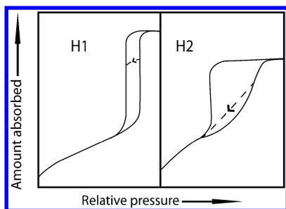
**Figure 7.** Examples of ideal desorption hysteresis scanning isotherms for Type H1 and Type H2 hysteresis. In Type H1 hysteresis, the scanning isotherm goes across the hysteresis loop. In Type H2 hysteresis, the scanning isotherm joins the desorption boundary isotherm at the lower closure point of hysteresis.
