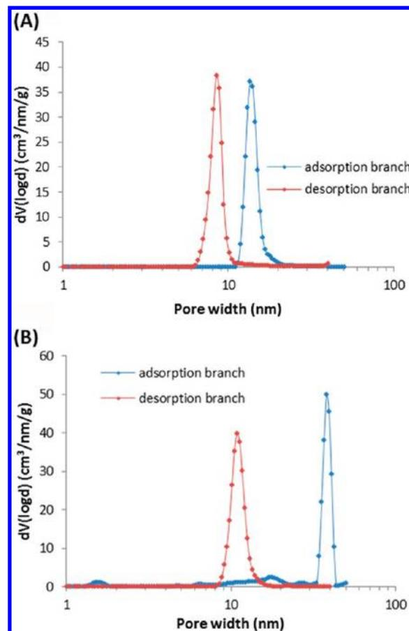
**Figure 6.** Pore size (cavity size) distributions calculated from the adsorption and window size from the desorption branches of the  $N_2$  (77.4 K) isotherms for the (A) 10 nm 3DOm carbon and (B) 40 nm 3DOm carbon.
