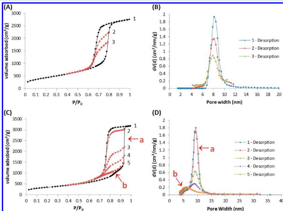
**Figure 8.** (A) Argon desorption scanning curves for the 10 nm 3DOM carbon, (B) distributions of the maximum neck size calculated from the desorption scanning curves for the 10 nm 3DOM carbon, (C) desorption scanning curves for the 40 nm 3DOM carbon, and (D) distributions of the maximum window size calculated from the desorption scanning curves for the 40 nm 3DOM carbon.
