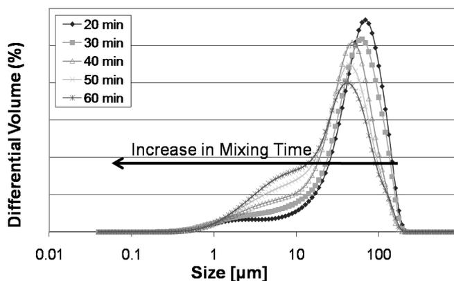
Fig. 7: Particle size distribution as a function of time for 1% acid.
