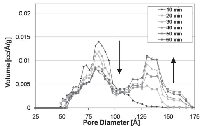
Fig. 4: Pore size distribution as a function of mixing time for 1% acid.
