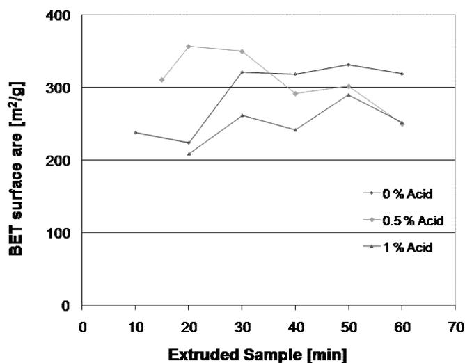
Fig. 1: BET surface areas results for the extruded samples as a function of mixing time.
