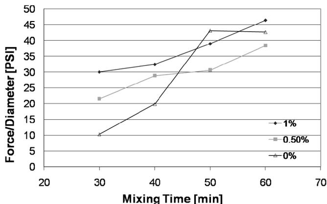
Fig. 5: Crush strength as a function of mixing time.
