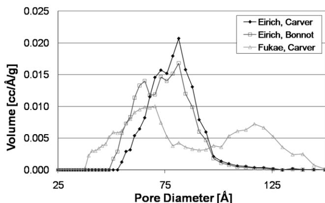
Fig. 8: Pore size distribution for pastes mixed and extruded by two different methods. The first term in parentheses signifies the type of mixer used, while the second term signifies the type of extruder used.
