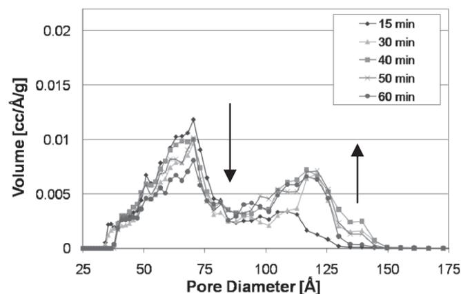
Fig. 3: Pore size distribution as a function of mixing time for 0% acid.
