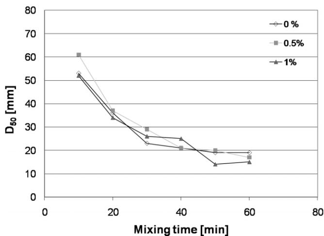
Fig. 6:  $D_{50}$  particle size values for the granulated samples as a function of mixing time for 0%, 0.5% and 1% acid case.
