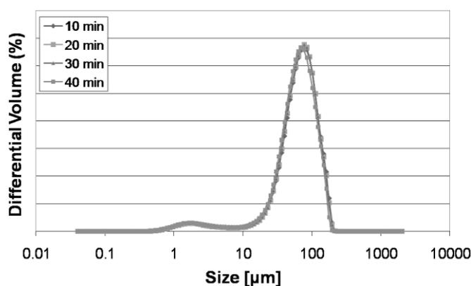
Fig. 9: Particle size distribution as a function of time for pastes prepared via Eirich mixer.
