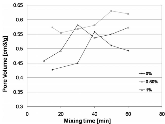
Fig. 2: Total pore volume results for the extruded samples as a function of mixing time.
