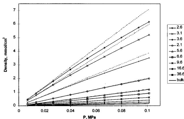
**Figure 3.** NLDFT absolute adsorption isotherms of He in carbon micropores at 77.4 K. The density of He has been calculated from eq 39. Dotted lines are Henry isotherms. Pore sizes are internal,  $H_{\text{in}}$ .
