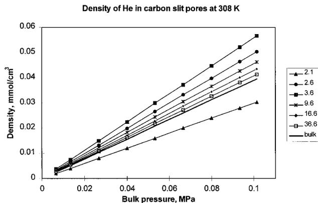
**Figure 7.** NLDFT absolute adsorption isotherms of He in carbon micropores at 308 K. The density of He has been calculated from eq 39. Pore sizes are internal,  $H_{\text{in}}$ .
