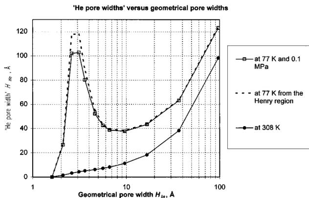
**Figure 6.** He calibrated pore widths,  $H_{\text{He}}$  (eq 43), versus the geometrical (internal) pore widths,  $H_{\text{in}}$ . Dotted lines are He pore widths calculated from the Henry region,  $H_{\text{He,Henry}}$  (eq 44), at 77 K. At 308 K,  $H_{\text{He}}$  is identical to  $H_{\text{He,Henry}}$ .
