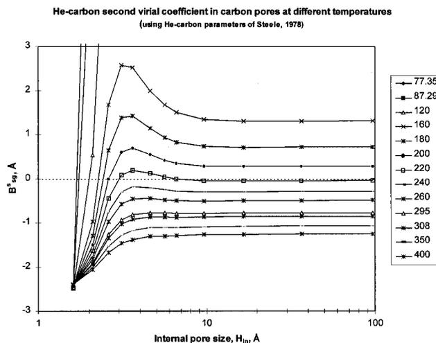
**Figure 5.** Solid–gas second virial coefficients of He in carbon slit pores at different temperatures. Calculated from eq 42. In the bottom half, the region around  $B_{sg}^s = 0$  is expanded. Temperature in Kelvin.
