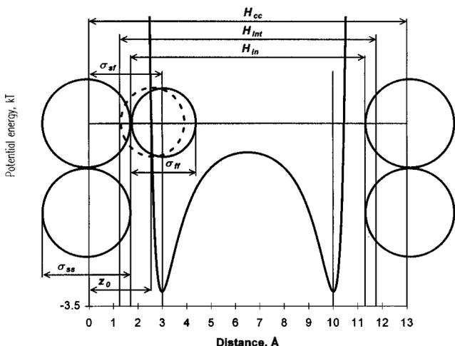
**Figure 2.** Various definitions of the pore size on the example of He in a carbon slit pore. 10-4-3 potential of Steele. He-carbon parameters were taken from combining rules (see text).
