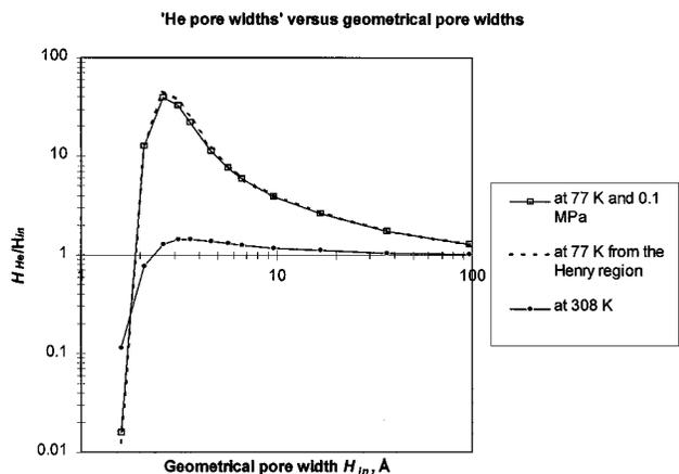
**Figure 4.** Ratio of the He calibrated pore widths,  $H_{He}$  (eq 43), to the geometrical (internal) pore widths,  $H_{in}$ . Dotted lines are He pore widths calculated from the Henry region,  $H_{He,Henry}$  (eq 44), at 77 K. At 308 K,  $H_{in}$  is identical to  $H_{He,Henry}$ .
