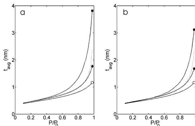
Fig. 5. Predicted amount of nitrogen adsorbed on a collection of touching spheres (a), and on a collection of merging spheres with  $m = 2$  nm (b). The data are normalized by the geometrical free surface of the spheres, so that it is an average thickness of the adsorbed film. The dotted line is the standard isotherm used for the calculations (FHH2); (○) is an isolated sphere ( $N_C = 0$ ); (◆) is for  $N_C = 2$ ; (■) for  $N_C = 12$  in (a) and  $N_C = 5$  in (b).
