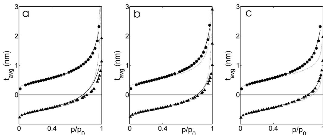
Fig. 7. Experimental average thickness of the film adsorbed on aerogels AT05 (●) and AT40 (▲) determined as explained in the text, using standard isotherms FHH1 (a), FHH2 (b) and LiC (c). The symbols are the experimental values, the dotted line is the standard isotherm, and the solid line is the best fit of the data with Eq. (17) with only the coordination number as adjustable parameter. On each graph, the two samples were arbitrarily shifted vertically.
