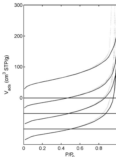
Fig. 2. Nitrogen adsorption (solid line) and desorption (dotted line) isotherms of aerogels AT05, AT15, AT25 and AT40 (from top to bottom). The data were arbitrarily shifted vertically.
