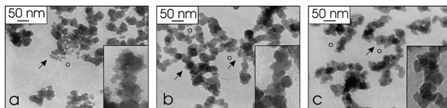
Fig. 1. Example of TEM micrographs of fragments of samples AT025 (a), AT05 (b), and AT40 (c). The circles drawn in the images have a diameter of 15 nm, representative of the particles from which the filaments are made up (arrows). The insets are magnified views of the same samples.
