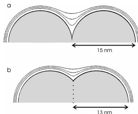
Fig. 4. Example of two touching spheres of diameter 15 nm, and the calculated free surface of the adsorbed film at  $P/P_0 = 0.4, 0.8$  and  $0.95$ , from Eq. (8). In (a) the spheres are simply in contact, and in (b) the spheres overlap by  $m = 2$  nm. The standard isotherm used for the calculation is FHH2.
