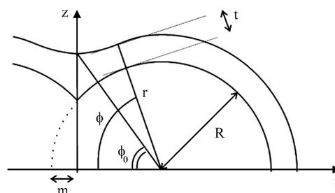
Fig. 3. Coordinates used to analyze the adsorption on two touching spheres and meaning of some symbols.  $(r, \phi)$ : spherical coordinates,  $R$ : radius of the spheres,  $m$ : degree of merging of the spheres,  $t$ : thickness of the adsorbed film.
