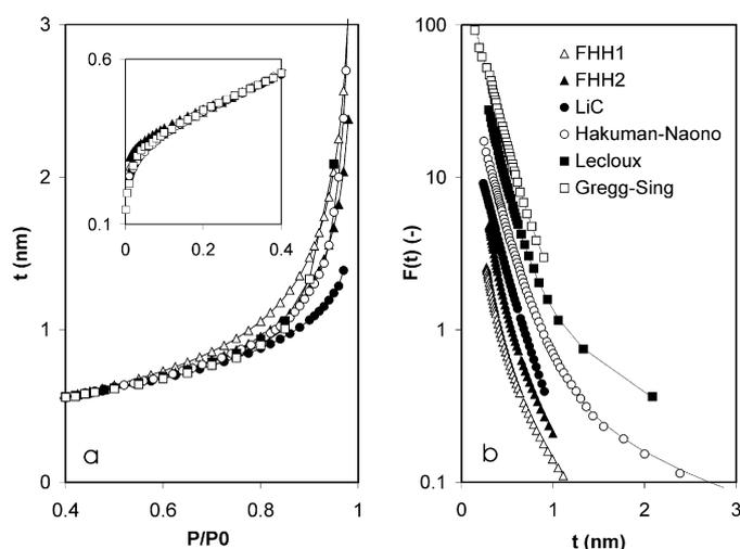
Fig. 6. Comparison of some standard isotherms reported in the literature for nitrogen adsorption on silica, in (a) under the form  $t(P/P_0)$  and in (b) under the equivalent form  $\ln(P/P_0) = F(t)$ : FHH1 [9], FHH2 [6,7,16], LiC [17], Hakuman–Naono [18], Lecloux [2], Gregg–Sing [14]. The inset in (a) is the low pressure part of the standard isotherms; in (b) the curves are shifted vertically; the solid lines are the fits of  $F(t)$  with Eq. (18) together with the parameters given in Table 1.
