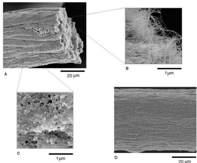
Fig. 1. Hierarchical pore structure morphology of CNF threads. (A) Tip of a CNF thread of about 50  $\mu\text{m}$  in diameter produced with PVA solution. (B) Highly porous nanofelt formed of SWCN bundles of 5–30 nm in diameter. (C) Porous mesh structure on the external surface is composed of polymer-bound SWCN bundles. (D) External surface of fibers produced with PVA/ethanol solution is less corrugated.
