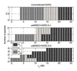
Figure 8: Number of correct codewords,  $m_c$ , detectable erroneous codewords,  $m_d$ , and undetectable erroneous codewords,  $m_{ud}$ , at the output of the decoder for different underwater MIMO designs in comparison with conventional HARQ.
