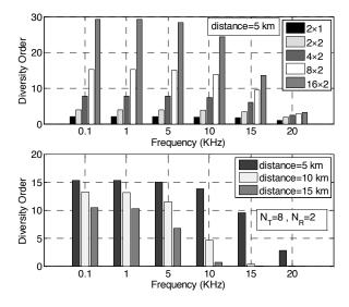
Figure 7: Effect of frequency and link distance on the performance of the system for a fixed distance and varying number of antennae (upper sub-figure) and for a fixed number of antennae at different distances (bottom sub-figure).
