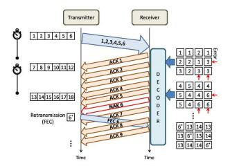
Figure 3: Proposed uwMIMO-HARQ type-II selective repeat scheme to reduce the probability of retransmission, where received packets and their copies are shown at the receiver. Here, packets 3 and 6 are erroneous; however, packet 3 has an acceptable copy and passes the error control process, whereas packet 6 is detected as erroneous and needs retransmission.
