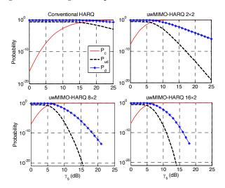
Figure 11: Probabilities of correct reception,  $P_c$ , of detecting error,  $P_d$ , and of undetectable error,  $P_{ud}$ , in different underwater MIMO designs and in conventional HARQ.
