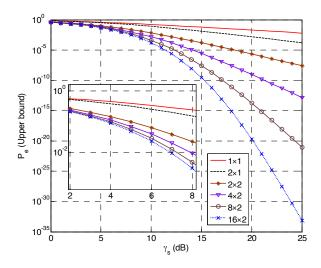
Figure 5: Average symbol error rate vs. Signal-to-Noise Ratio (SNR) for different numbers of antennae in an underwater MIMO system.
