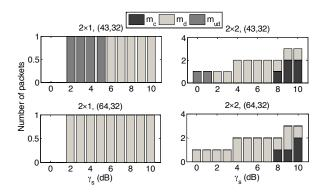
Figure 12: Waterfilling technique for low SNR regimes for different MIMO designs when two Reed-Solomon codes are used, i.e., (43,32) and (64,32).
