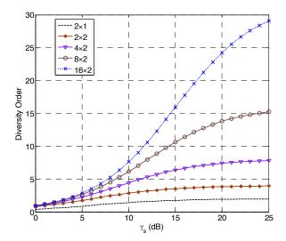
Figure 6: Diversity order vs. SNR for different numbers of antennae. Well-conditioned channel regime is the range of high SNRs where the diversity order approaches the value of  $N_T N_R$ . Ill-conditioned regime is the range of SNR in which the diversity order drops.
