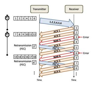
Figure 2: Conventional HARQ type-II selective repeat scheme, where packets are labeled with ID numbers and  $\star$  denotes the extra data to implement Forward Error Correction (FEC) of previous packet at the receiver. A timer keeps the round-travel time and triggers a retransmission if a time-out occurs. Here, packets 3 and 6 are erroneous and the transmitter is instructed via a NAK to retransmit the required information.
