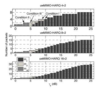
Figure 9: Number of correct codewords,  $m_c$ , detectable erroneous codewords,  $m_d$ , and undetectable erroneous codewords,  $m_{ud}$ , for different underwater MIMO designs with a large number of transmitted antennae. Different channel conditions are presented in the top sub-figure.
