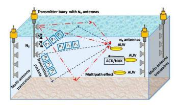
Figure 1: Configuration of the proposed MIMO system, where  $N_T$  and  $N_R$  are the number of transmit and receive antennae, respectively,  $P_i's; \forall i=1,2,3,...$  are the coded transmitting packets, and ACK/NAK denotes positive or negative acknowledgements of the reception of a packet.
