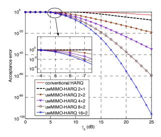
Figure 10: Acceptance error,  $\mathcal{E}_a$ , of our uwMIMO-HARQ (using different settings) in comparison with conventional HARQ.
