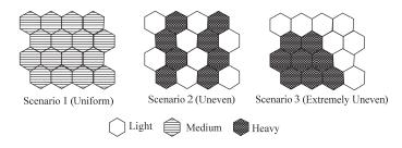
Fig. 3. Different user distribution scenarios: Scenario 1 (uniform) with all *medium* (loaded) cells; Scenario 2 (uneven), *light* and *heavy* (loaded) cells are intermixed together; Scenario 3 (extremely uneven), *heavy* cells are grouped together, and the heavy cell group is surrounded by *light* cells.
