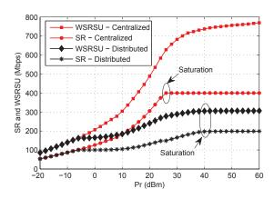
Fig. 5. Downlink WSRSU of a C-RAN system with centralized computing resource (*Centralized*) versus that of a traditional system with distributed computing resources (*Distributed*).
