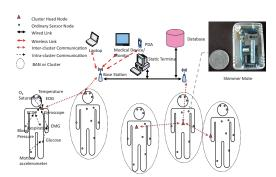
Fig. 1. Proposed Physical Network Architecture.
