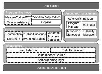
Fig. 1: CometCloud system architecture
