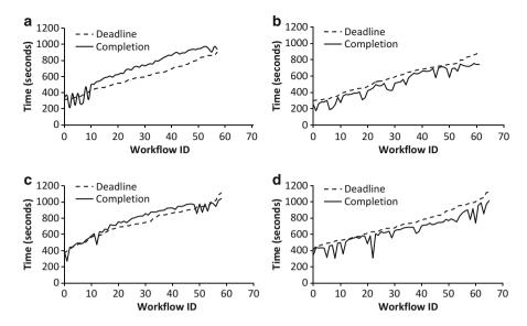
**Fig. 8** Deadline and completion time of each workflow with and without cloudburst. (**a**) Only Rutgers (No Cloudburst), deadline 300 s. (**b**) Rutgers+EC2 (CloudBurst), deadline 300 s. (**c**) Only Rutgers (No Cloudburst), deadline 420 s. (**d**) Rutgers+EC2 (CloudBurst), deadline 420 s
