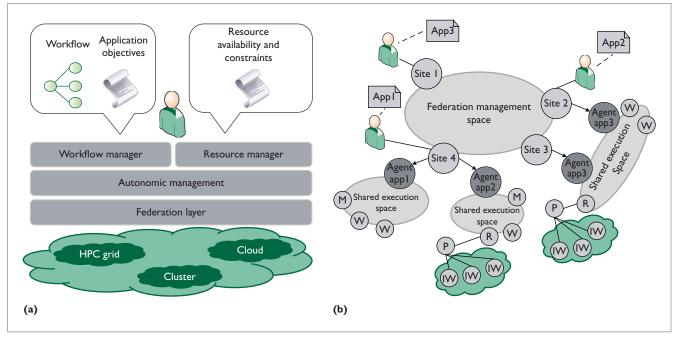
Figure 1. CometCloud. (a) The CometCloud architecture comprises three key layers: infrastructure/federation, autonomic management, and programming/interface. (b) The CometCloud coordination model is used to orchestrate different aspects of the federation.
