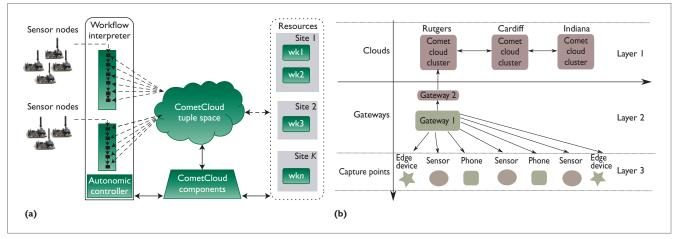
Figure 3. CometCloud use cases in the smart infrastructure domain. We can see the architectures for the (a) streaming data<sup>7</sup> and (b) building analytics<sup>8</sup> use cases.
