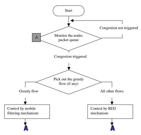
Figure 4.2 Flowchart for high level design of our congestion control algorithm
