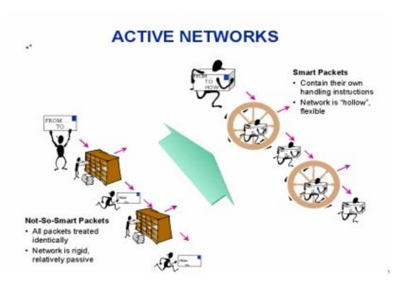
Figure 1.1 Comparing traditional networks with active networks
