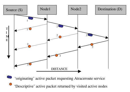
Figure 4.1 Operation of Atraceroute
