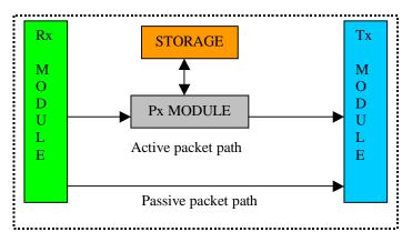
Figure 3.1 High-level design of the active node
