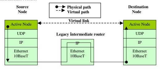
Figure 3.5 Movement of packets in the RANI network
