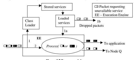
Figure 3.7 Process module
