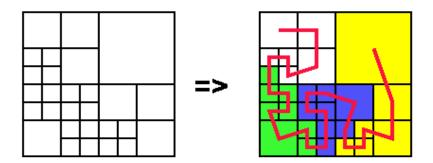
Figure 3.1 Space-Filling Curve Representation of an Adaptive Grid Hierarchy
