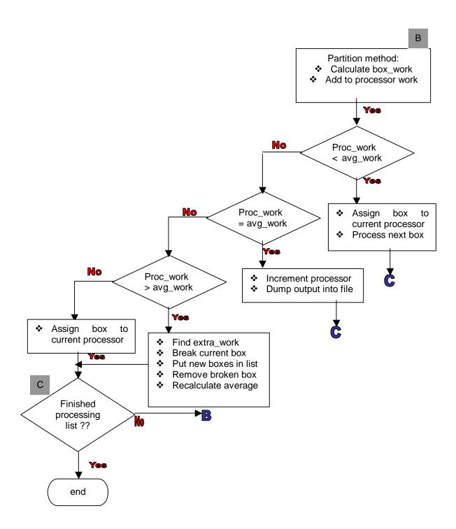
Figure 4.7 Flow Diagram FD1 (Continued ...): Original Partition Method
