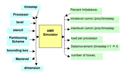
Figure 5.2 Inputs and Outputs to the Simulator
