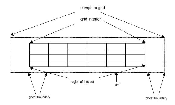
Figure 2.2 Components of a Grid
