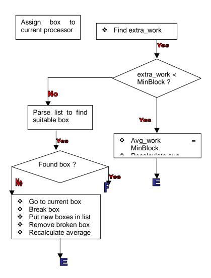
Figure 4.10 Flow Diagram FD2 continued..: Optimized Partition Method
