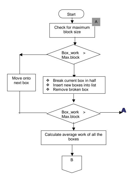
Figure 4.6 Flow Diagram FD1: Original Partition Method
