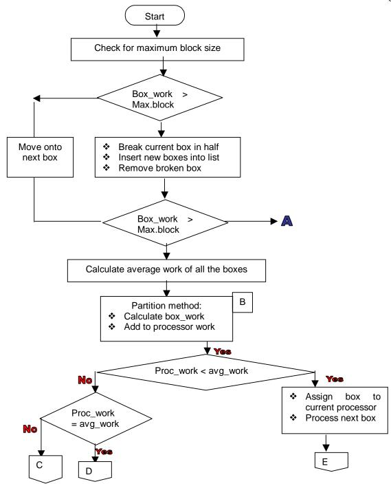
Figure 4.9 Flow Diagram FD2: Optimized Partition Method
