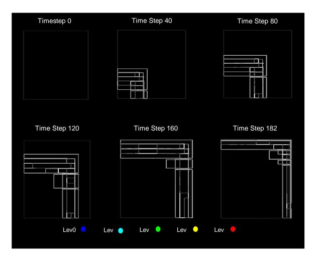
Figure 1.1 AMR Grid Structure for Buckley-Leverette Application
