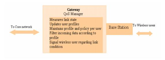
Figure 3.4 Wireless gateway QoS Manager Functions
