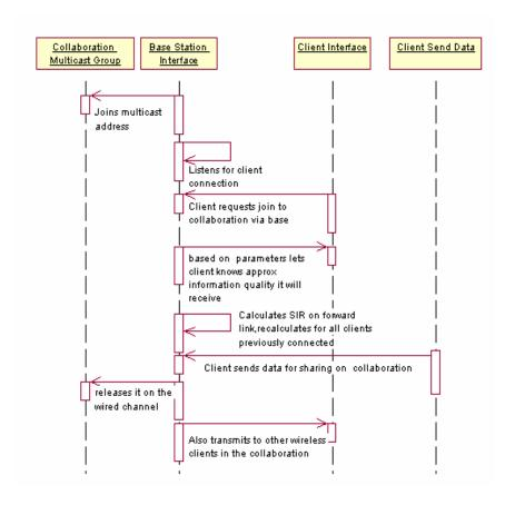
Figure 5.3 Interaction diagram in SIM Application
