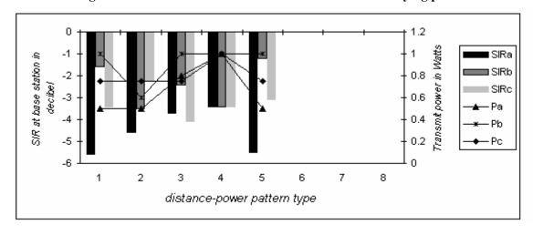
Figure 5.6 Performance of 3 wireless clients with varying distance and power
