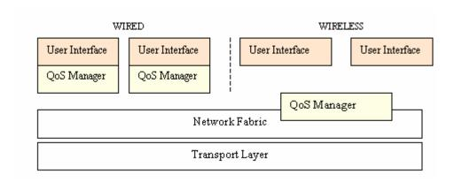
Figure 3.3 QoS Manager in Heterogeneous Collaboration Framework
