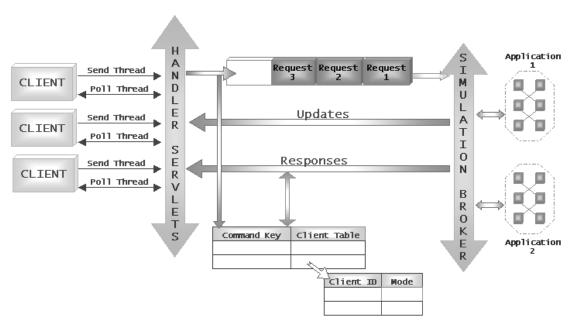
Figure 6: - Client Server Communication Model in DISCOVER
