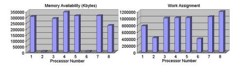
**Figure 3.** Lightly loaded scenario on 8 processors: Memory availability (left) and work assignment for memory-based proactive partitioning algorithm (right)
