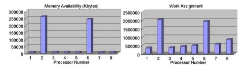
**Figure 5.** Heavily loaded scenario on 8 processors: Memory availability (left) and work assignment for memory-based proactive partitioning algorithm (right)
