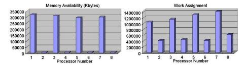
**Figure 4.** Moderately loaded scenario on 8 processors: Memory availability (left) and work assignment for memory-based proactive partitioning algorithm (right)
