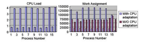
Figure 2. Moderately loaded scenario on 16 processors: CPU load distribution (left) and work assignment for 16 processors (right)
