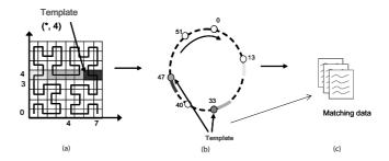
Figure 5: Example of tuple retrieval in Comet: (a) the template defines a rectangular region in the 2-dimensional space consisting of 3 clusters; (b) the nodes that store the clusters are queried; (c) results of the query are sent to the requesting node.
