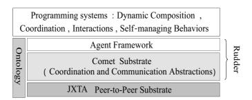
Figure 1 A conceptual overview of Rudder.
