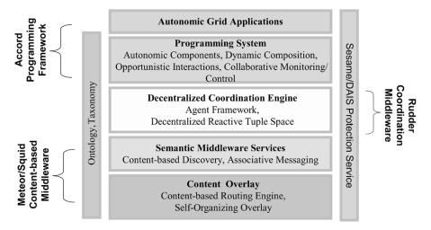
Fig. 4. A schematic overview of AutoMate.
