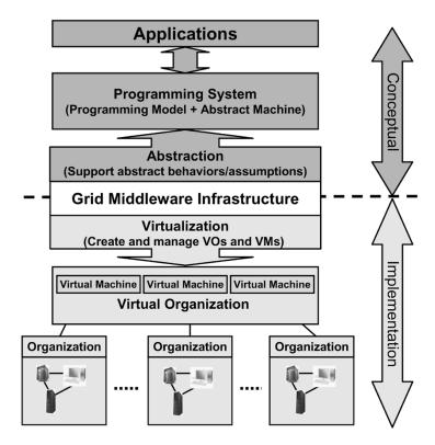
Fig. 1. Conceptual and implementation models for Grid computing.
