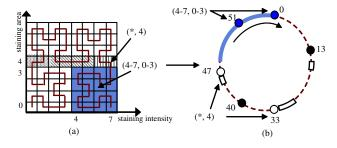
Figure 10. Processing the query (\*, 4): (a) the query defines a rectangular region in the 2-dimensional keyword space, and 3 clusters (3 segments on the SFC curve); (b) the clusters (the solid part of the circle) are stored at nodes 33 and 47, so these nodes will be queried.
