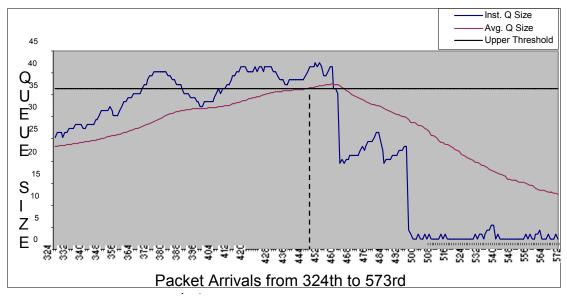
Figure 8 – Plot of queue size v/s packet at Node I3
