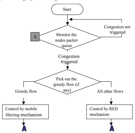
Figure 1 – An overview of the LGC Congestion Control Mechanism
