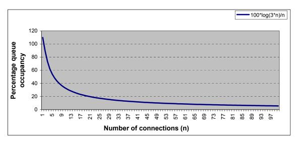
Figure 2 – Percentage of permissible queue occupancy (qo) v/s number of connections (n)
