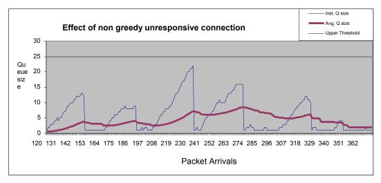
Figure 6 – Plot of queue size v/s packet arrivals for non-greedy connections
