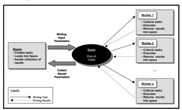
Figure 2 – Master-Worker Parallel Computing using JavaSpaces
