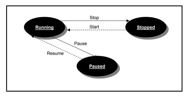
Figure 5 - Worker State Transition Diagram
