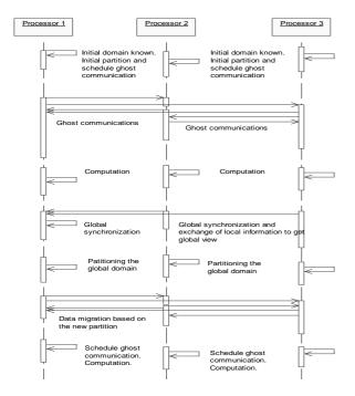
Figure 2. Sequence diagram of the Non-HPA scheme
