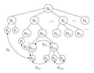
Figure 3. A general hierarchical structure of processor groups
