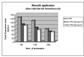
Figure 5. Execution time: Static HPA versus Non-HPA scheme
