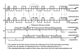
Fig. 1. Timing Diagram for Parallel SAMR Algorithm
