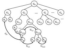
**Fig. 4.** A General Hierarchical Structure of Processor Groups
