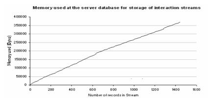
Figure 5. Graph showing memory usage by Interaction Streams
