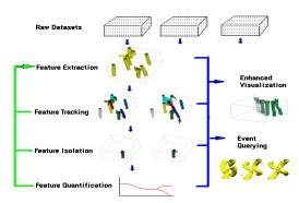
Figure 1. A process for visualizing 3D continuum datasets
