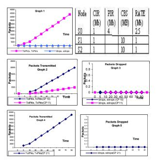
Figure 3: Out-of-profile S0 gets downgraded not affecting in-profile S1 and S2
