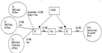
Figure 2: Topology (A mixture of one EF and two AF flows)
