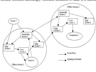
Figure 1: Test Network with Different Scenarios
