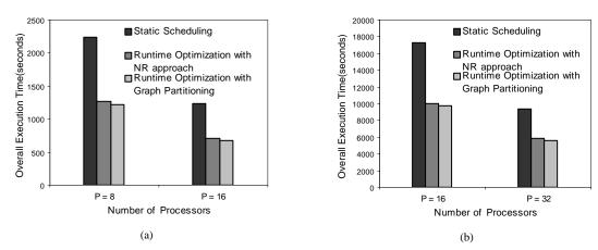
Figure 6. Overall performance of different optimization approaches on different processor configurations. (a) Problem size 65536 cells. (b) Problem size 262144 cells.
