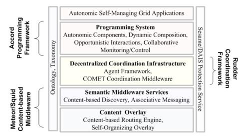
Fig. 1. A schematic overview of AutoMate
