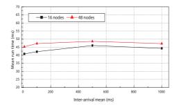
Fig. 6. Average round trip time for the Out operation for different mean inter-arrival time
