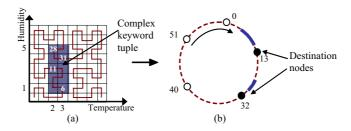
**Fig. 4.** Routing using a complex keyword tuple (2-3, 1-5): (a) the keyword tuple defines a rectangular region in the 2-dimensional keyword space consisting of 2 clusters (2 segments on the SFC curve); (b) the clusters (the solid part of the circle) correspond to destination RP nodes 13 and 32, which are routed to
