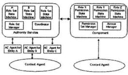
Fig. 7 Dynamic Access Control in AutoMate
