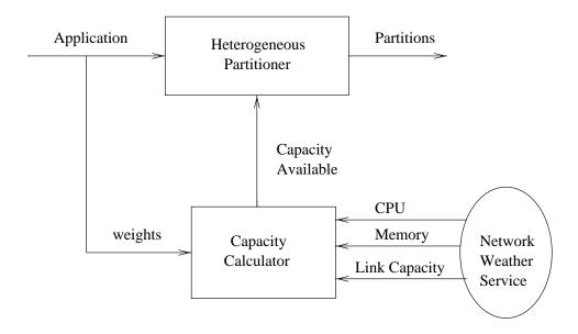
Figure 1: Block Diagram of the System Model
