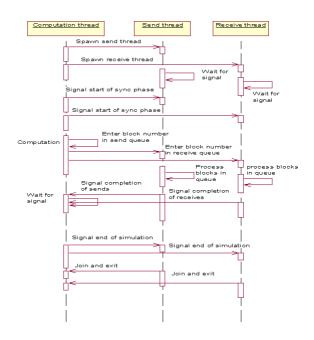
Figure 3: Sequence of events in the multithreaded engine on a single process
