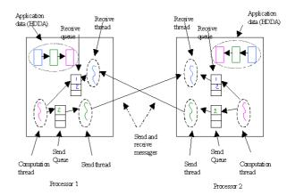
Figure 2: Architecture of the Multithreaded Communication Engine
