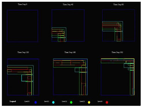
Figure 3. AMR Grid Structure (2D Example)
