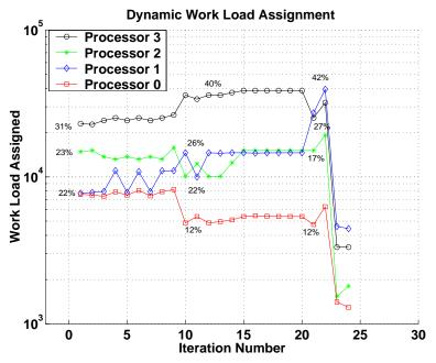
Figure 15. Dynamic load allocation for a system state sensing frequency of 40 iterations
