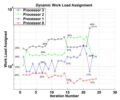
Figure 14. Dynamic load allocation for a system state sensing frequency of 30 iterations
