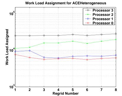
Figure 9. Work-load assignments for the ACEHeterogeneous partitioning scheme (Relative capacities of processors 0-3 equal to 16%, 19%, 31%, and 34% respectively).
