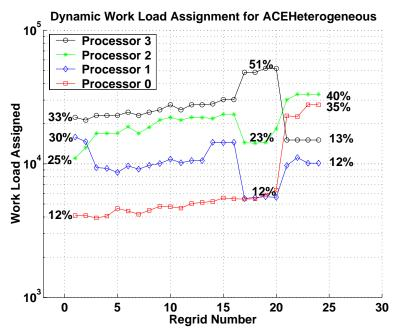
Figure 11. Dynamic load allocation using the system sensitive partitioner
