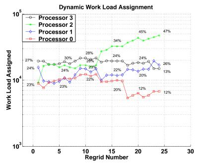
Figure 12. Dynamic load allocation for a system state sensing frequency of 10 iterations
