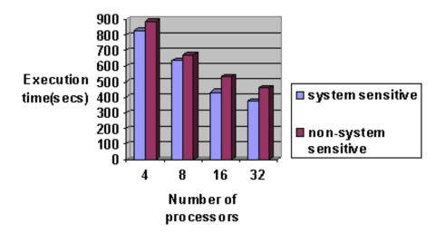
Figure 7. Application execution time for the system sensitive and default (non-system sensitive) partitioning schemes
