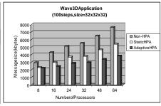
$\it Figure~6.$  Communication cost: comparison of Non-HPA, Static HPA and Adaptive HPA schemes
