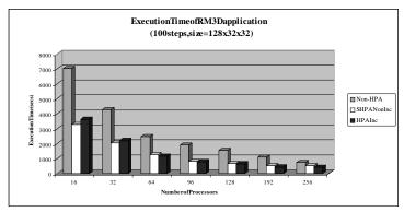
Figure 5. Execution time: Static HPA versus Non-HPA scheme
