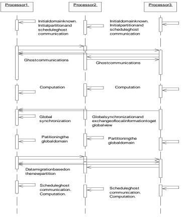
Figure 2. Sequence diagram of the Non-HPA scheme
