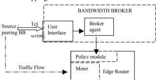
Fig:4 Modular breakup of BB and its interaction in traffic flow
