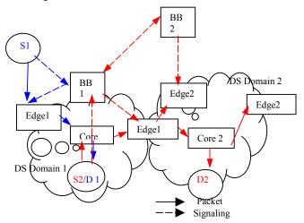
Fig3 Test network showing different scenarios
