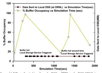
Figure 11 Effect of switching from the DSS at PPPL to the DSS ORNL in response to network congestion and/or failure.
