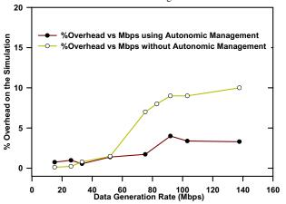
Figure 7(b). Percentage overhead on simulation execution with and without autonomic management.
