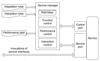
Figure 1. An autonomic service in Accord.
