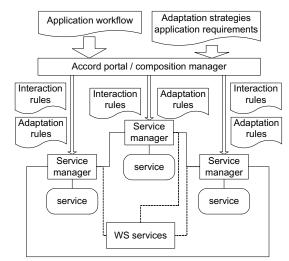
Figure 2. Accord runtime infrastructure. Solid lines indicate interactions among services and dotted lines represent invocation of WS instances providing supporting services such as naming and discovery.
