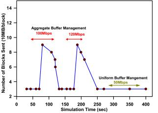
Figure 7(a). Self-optimization behaviors of the Buffer Management Service (BMS) – BMS switches between uniform blocking and aggregate blocking algorithms based on application data generation rates, network transfer rates and the nature of data generated.
