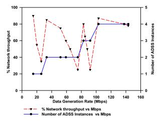
Figure 9. Effect of creating new instances of the ADSS service when the %Network Throughput dips to below the user defined 50% threshold.
