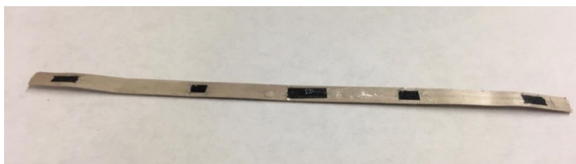
Fig. 3 HTS BSCCO tape used in the experiment
